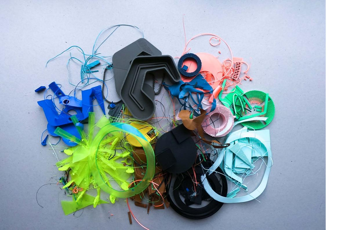
By-products and failed prints were collected and will be remade into new filament alongside the alarm prototypes.
