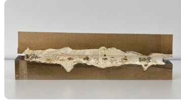
Mycelium is growing on hardwood with a rough surface. Both pieces were residual and have different dimensions.
