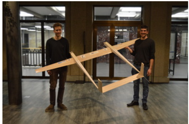
Leo Baumann and Cla Mattia Galliard pose with their custom-built prototype plane, dubbed LARA - Lightweight Autonomous Rope-Fixed Aircraft. The next incarnation, CLARA, will be made from carbon. (ftero)
