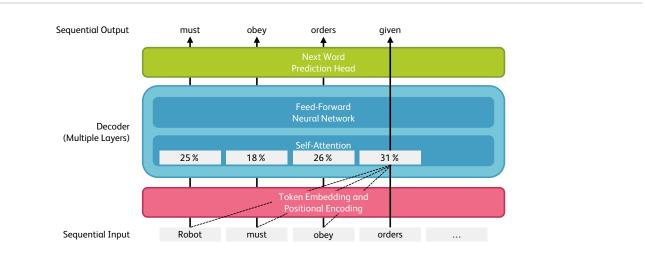
Figure 7.1: Simplified architecture of a generative pretrained transformer (GPT) (source: based on Alammar (2019))
